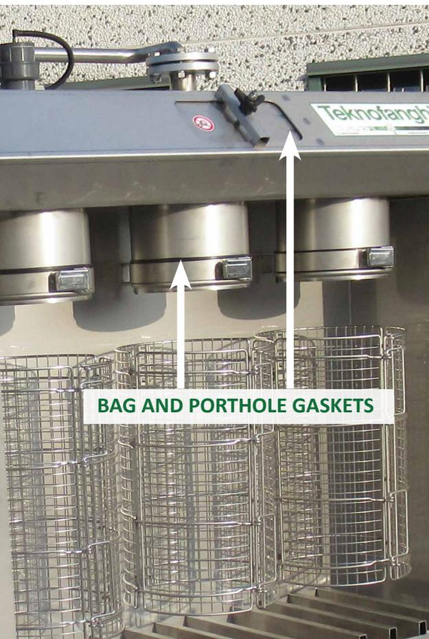
The most important gaskets we can find in a TEKNOBAG-DRAIMAD® unit are the **bag rubber gaskets** and the **rubber gasket for the upper inspection porthole**.
