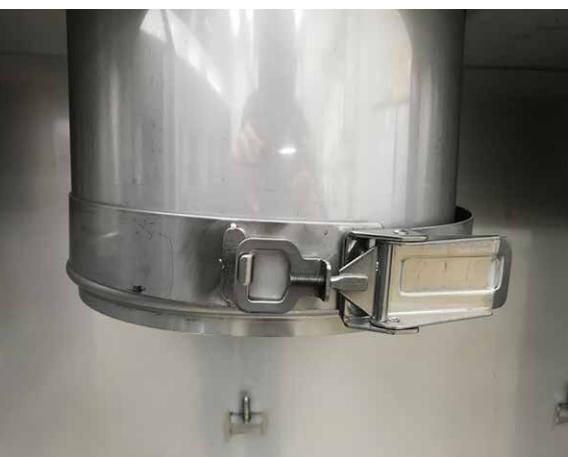
Over time, with the direct **contact with the sludge** and also with the **mechanical action** (constant opening and closing to change the bags), the **clamp can be damaged or**, in extreme cases, it can **break**.
