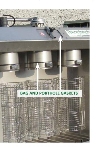
The most important gaskets we can find in a TEKNOBAG-DRAIMAD® unit are the **bag rubber gaskets** and the **rubber gasket for the upper inspection porthole.**
